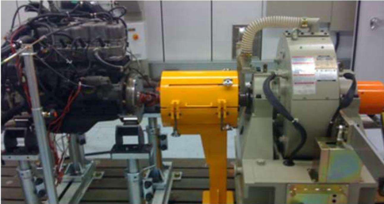
**Eddy current dynamometers** use a magnetic field to provide counter restraining torque that increases with shaft speed.
