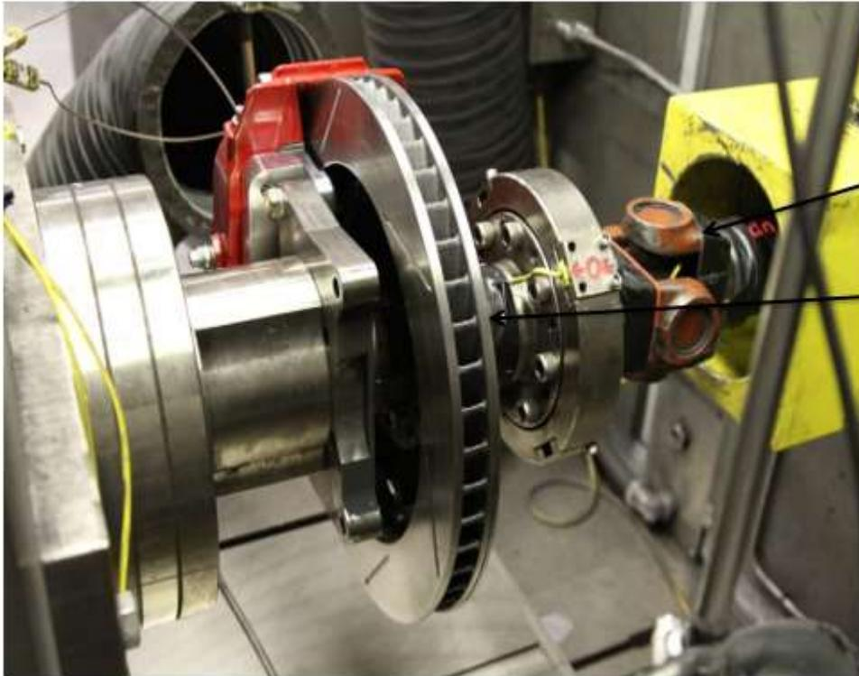
Prop shaft connects to flywheel of engine
