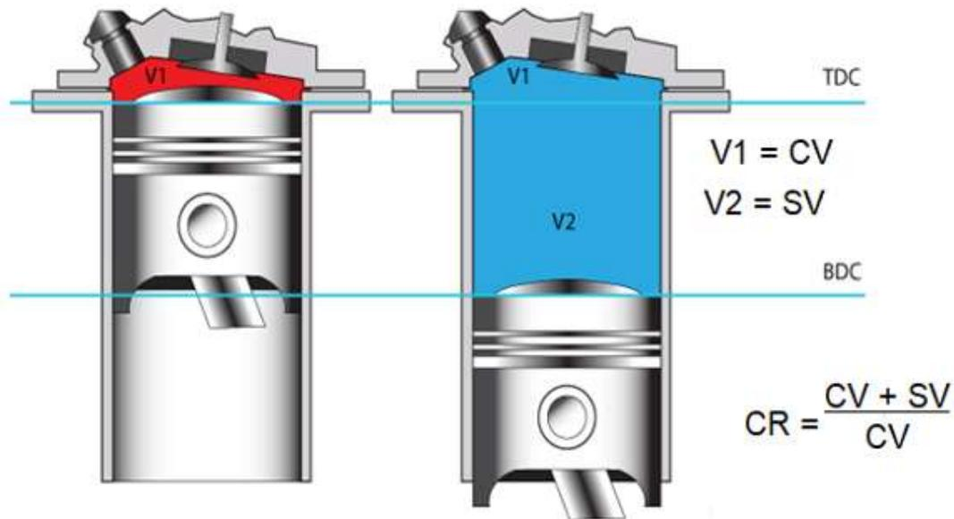
In other words, compression ratio is a comparison of the total volume of an engine cylinder (**swept volume + clearance volume**) when the piston is at BDC, to the volume of the cylinder when the piston is at TDC, **clearance volume**. Refer to the diagram above.
