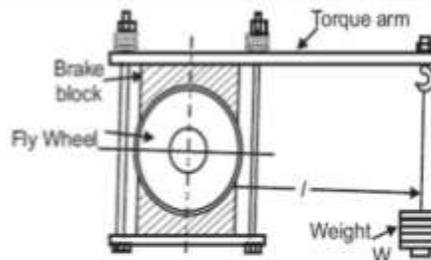
$$B.P. = \frac{\text{Work done per min.}}{60} = \frac{T \times 2\pi N}{60} = \frac{W \cdot l \times 2\pi N}{60} \text{ watts}$$
