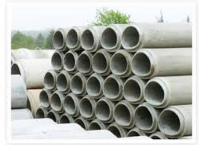
Concrete water pipes
